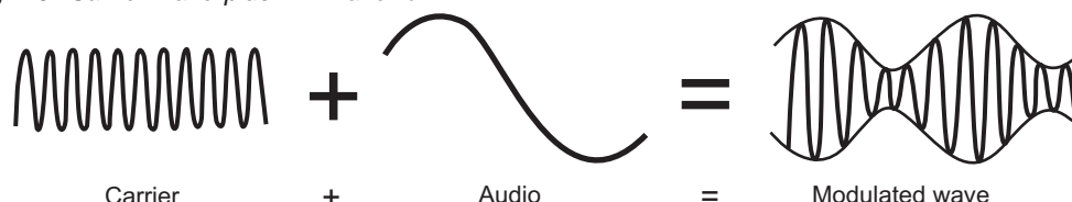
Fig 1-6: Carrier wave plus AM wave form
