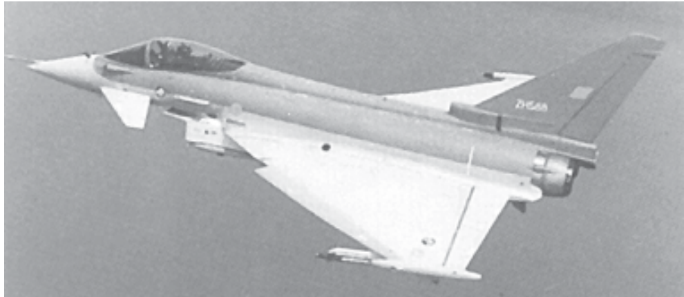
Fig 3-5 Delta Wing with Canard Foreplane (EF 2000)
