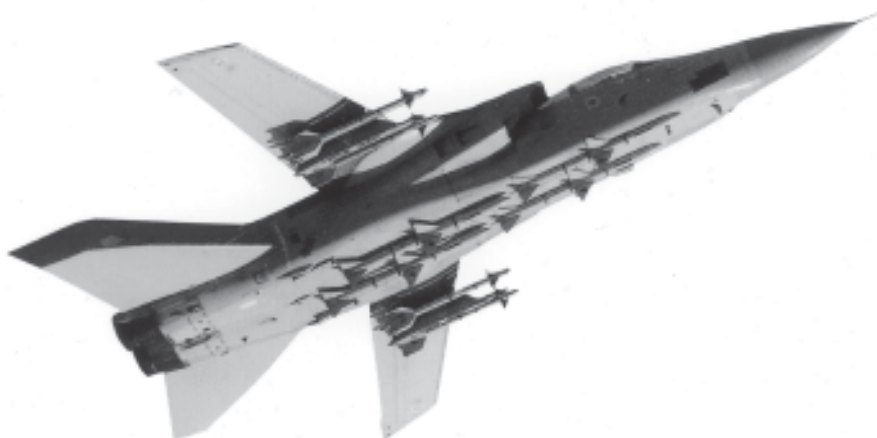
Fig 11-7 Tornado With Air-to-Air Missiles Skyflash and Sidewinder
