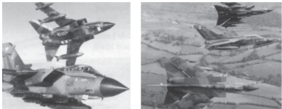
Fig 3-4 Variable Sweep-Back (Tornado)
